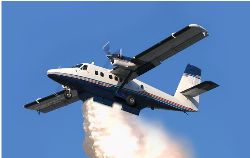
The photo is a mock-up of the DHC-6 Twin Otter Firefighter aircraft featuring the air tanker configuration.
