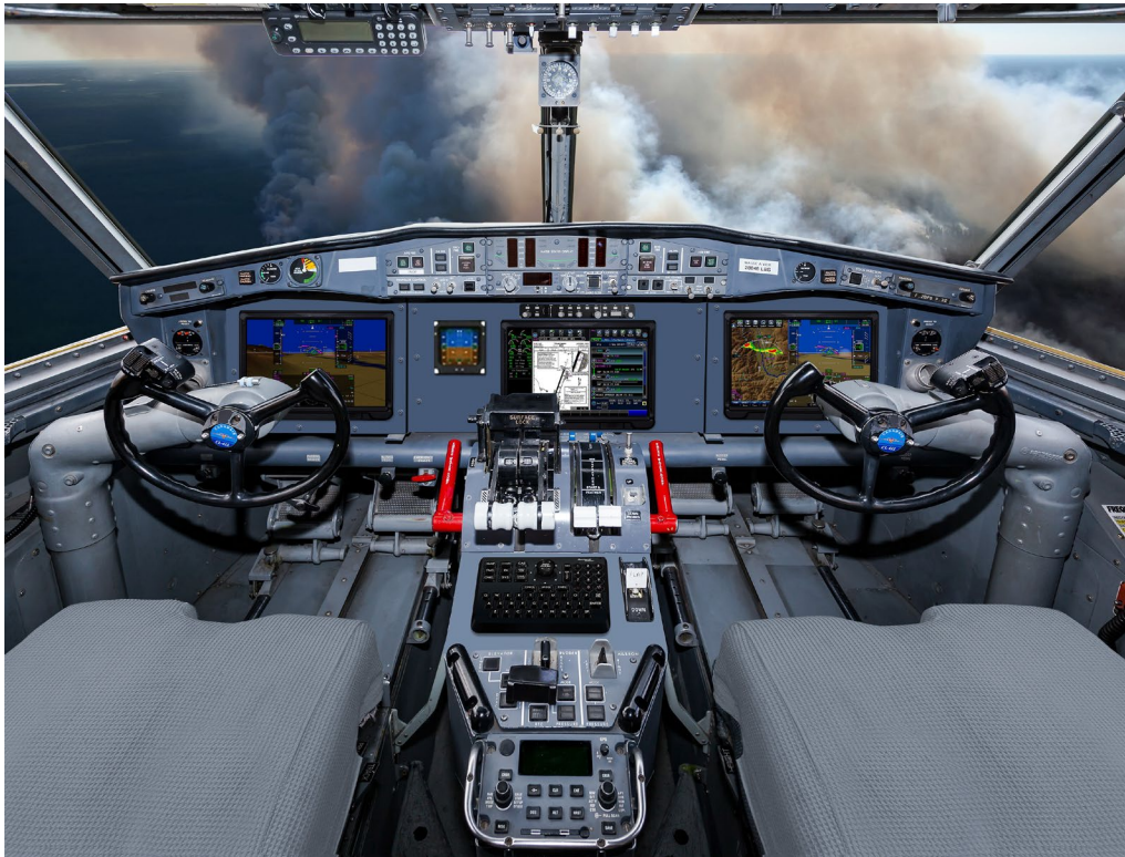
Pictured above: The proposed layout of the Collins Aerospace Pro Line Fusion integrated avionics suite to be featured in the Viking Avionics Upgrade Program (AUP).
