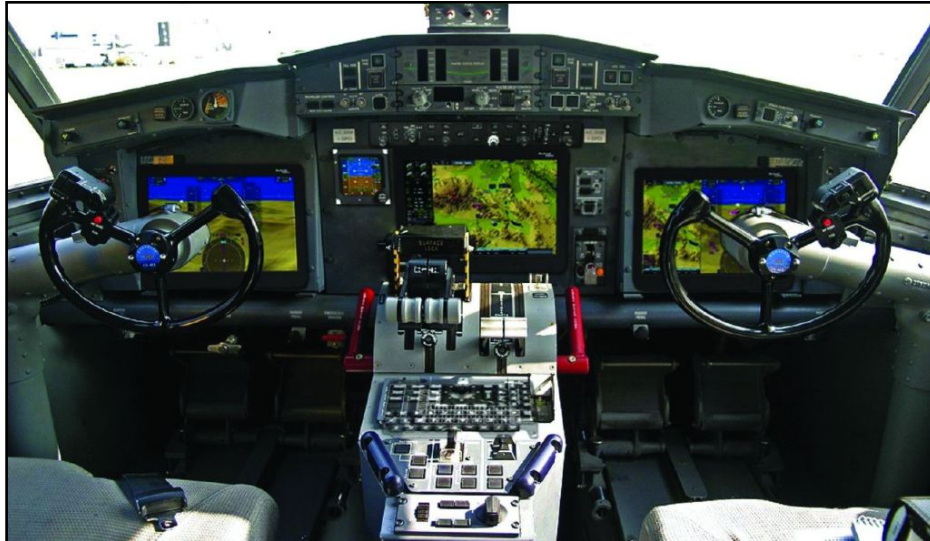
Pictured above: proposed layout of the Collins Aerospace Pro Line Fusion integrated avionics suite featuring 3-screen LCD displays.
