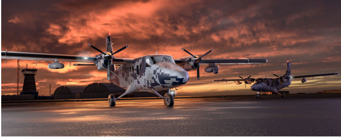
Pictured above: Artistic rendering of the Guardian 400 Technical Demonstrator aircraft, featuring R/H SCAR pod with Hensoldt Argos EO/IR imaging turret, L/H SCAR pod with Leonardo Osprey Radar System and Sentient Vidar Camera system, Airborne Technologies' tactical workstation, Viking conformal bubble windows, IKHANA L/H & R/H wing-mounted hard points, Thunder Bay Aviation stretcher racks, and aft lavatory.
