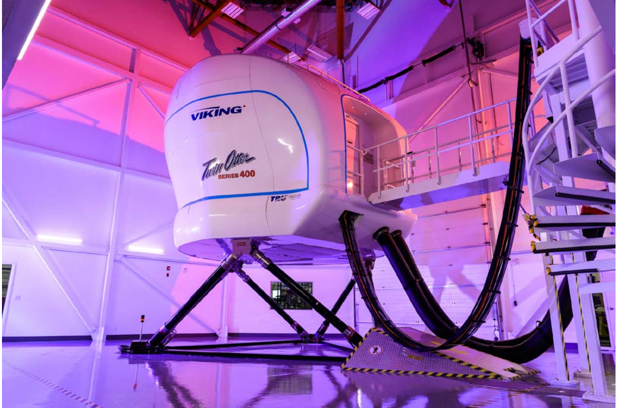
Approved by CAAC - Pacific Sky Aviation's Level D Series 400 Twin Otter Full Flight Simulator
