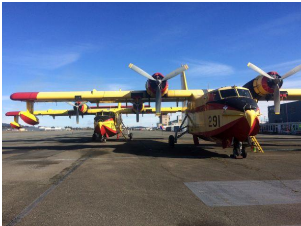
Pictured above: Two of Longview's eleven Canadair CL-215 aircraft that are destined for CL-415EAF Enhanced Aerial Firefighter Turbine Conversion, photographed on ramp at Viking Air Limited's facilities at Victoria International Airport.
