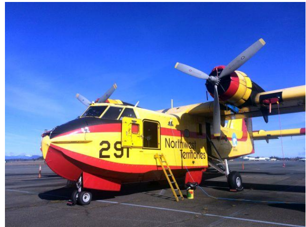
Pictured above: Two of Longview's eleven Canadair CL-215 aircraft that are destined for CL-415EAF Enhanced Aerial Firefighter Turbine Conversion, photographed on ramp at Viking Air Limited's facilities at Victoria International Airport.
