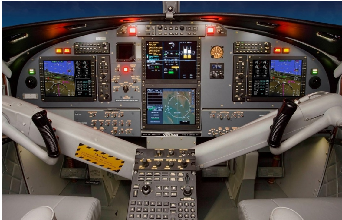
Pictured Above: the Honeywell Primus Apex fully-integrated digital avionics suite in the Viking Series 400 Twin Otter featuring Smartview synthetic vision system.
