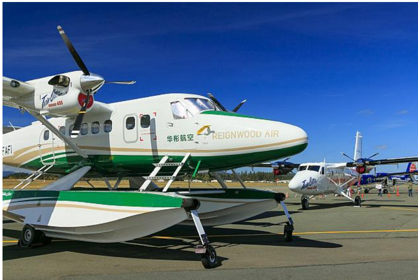
Pictured above: Reignwood Air's Series 400 Twin Otter equipped with Wipline® 13000 amphibious floats alongside Viking's 100 th production aircraft on the ramp at Viking's facility in Sidney, British Columbia.
