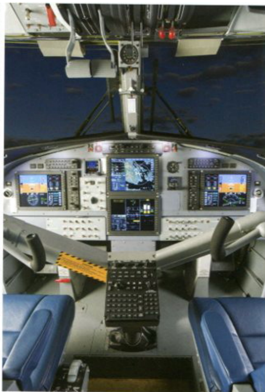
The glass cockpit installation in the Twin Otter series 400
