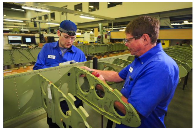
Pictured above: Viking employees install commemorative signed ribs into the wings of Viking's 100 th production Twin Otter Series 400 aircraft at the company's corporate headquarters in Victoria, British Columbia, Canada.
