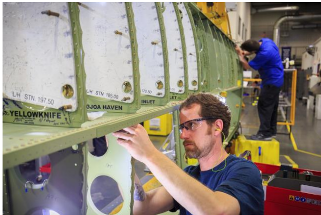
Pictured above: Viking employees install commemorative signed ribs into the wings of Viking's 100 th production Twin Otter Series 400 aircraft at the company's corporate headquarters in Victoria, British Columbia, Canada.
